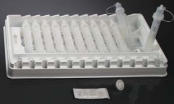
DispoRack ™ with 12 ITUs (Iron Testing Units)
